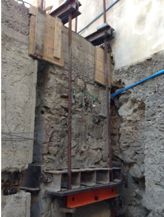
Figure 4. Test setup for panel in compression.
